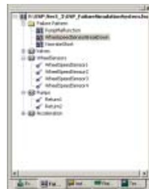
◀ The Failure Navigator in ControlDesk Failure Simulation: Central handling of failure simulation hardware, failure patterns and all ECU channels.
