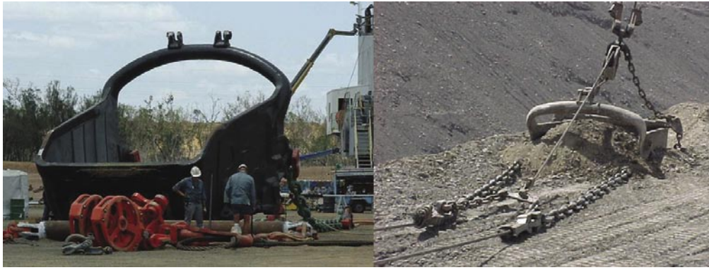
◀ The bucket for scooping up overburden: Weight 40 tons when empty, 120 tons when full.
