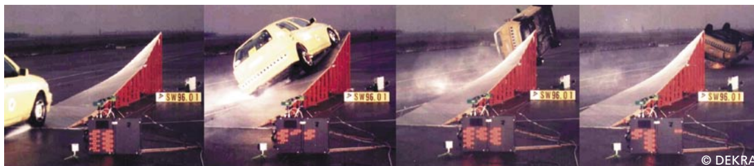
▲ In situations like these, the WinGAMR rollover detection algorithm triggers safety measures.
