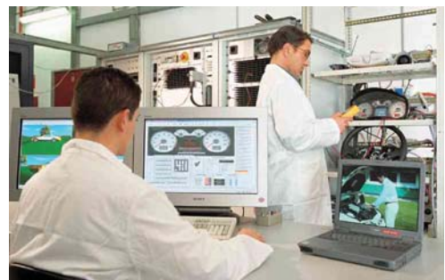
▲ ELASIS' virtual car: The networked simulators are controlled from one central PC.
