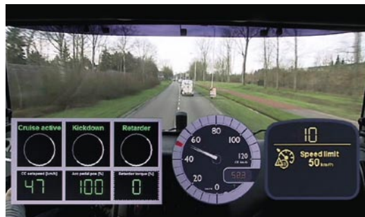
▲ To overtake, the driver overrules the Safe Speed Function.
