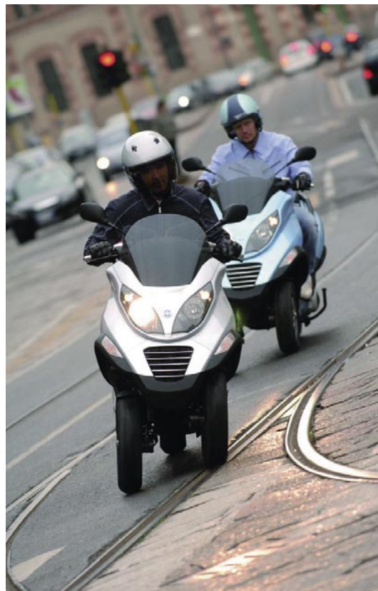
▲ The MP3 provides a tilt angle of up to 40°.
