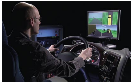
▲ The test driver has a real steering wheel and can see the truck's behavior on a screen.
