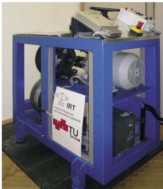
▲ Design of the test bench with MicroAutoBox and operating console.
