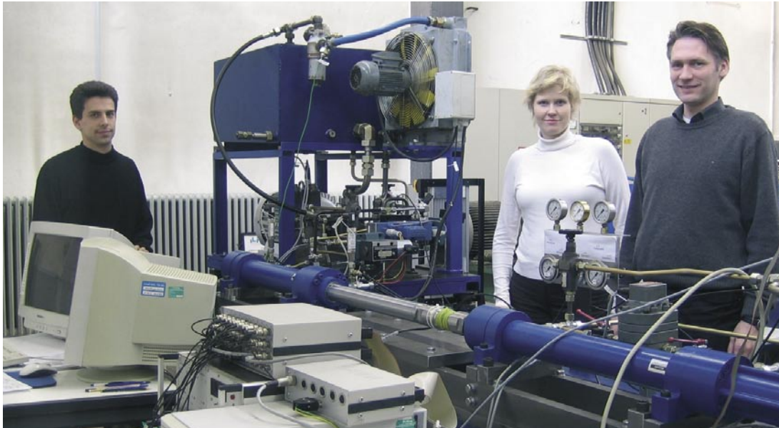
◀ The stationary test bench: The research team analyzes the effect of air in a working hydraulic system in a mobile working machine. From the left: Björn Grösbrink, Julia Lechnitz, Thomas Fedde.
