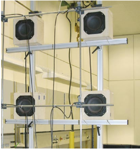
▲ Experimental setup of a loudspeaker-error microphone system for active noise reduction.
