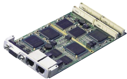
▲ The PMC Module AMC-FDX-2 for connection to the AFDX network.
