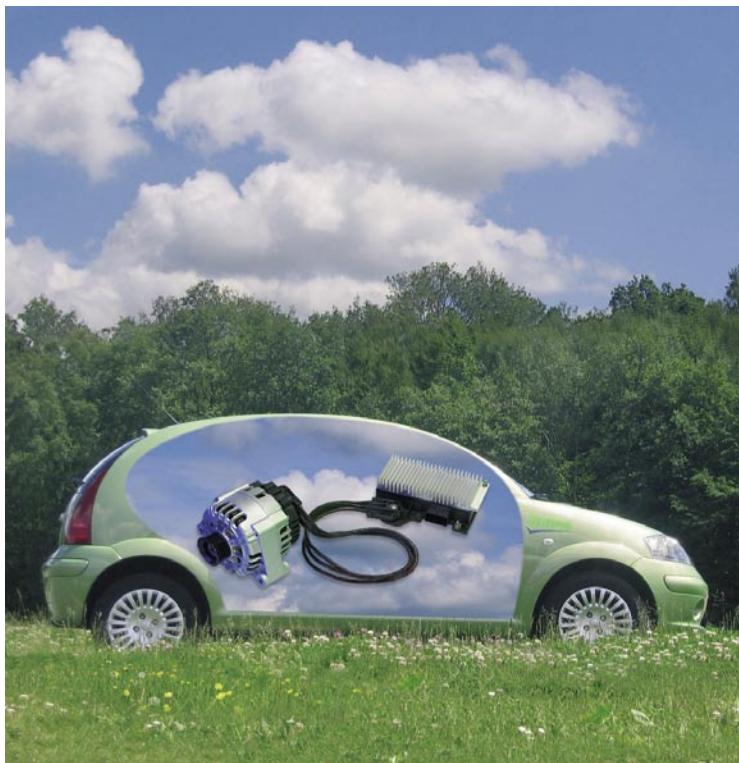
▲ The StARS micro-hybrid system: Electric machine, three-phase cable, and control box.
