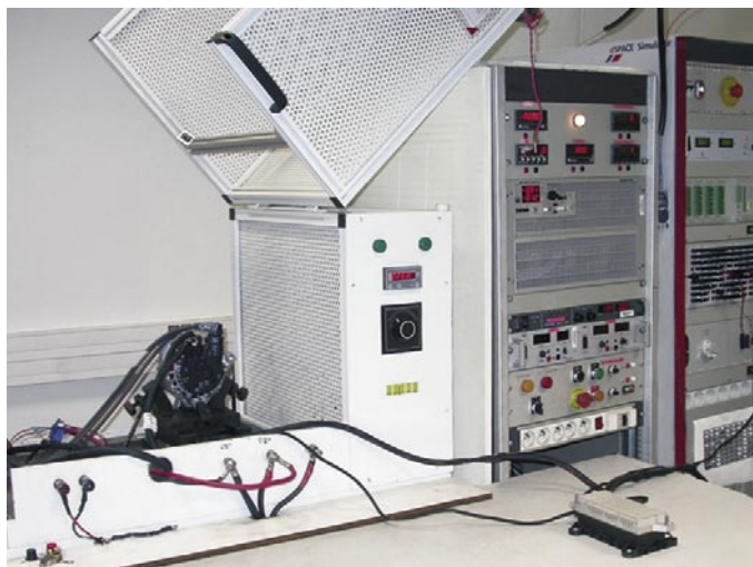
▲ The validation bench based on dSPACE Simulator Full-Size.
