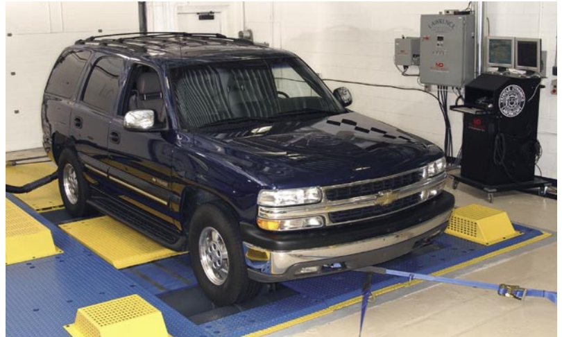
▲ Lawrence Tech’s four-wheel drive chassis dynamometer gives students an optimum platform for exploring innovative automotive engineering solutions.
