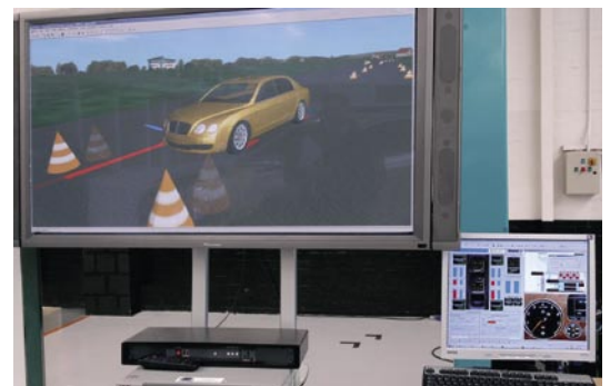
▲ MotionDesk visualized driving maneuvers during driver-in-the-loop tests.
