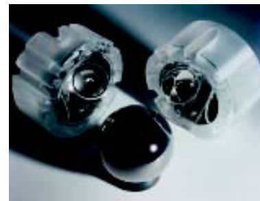
The gap between the rotor and the six suspension electrodes is less than 20 micrometers.
