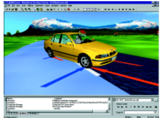
Vectors visualize the forces between the wheels and the road in MotionDesk.
