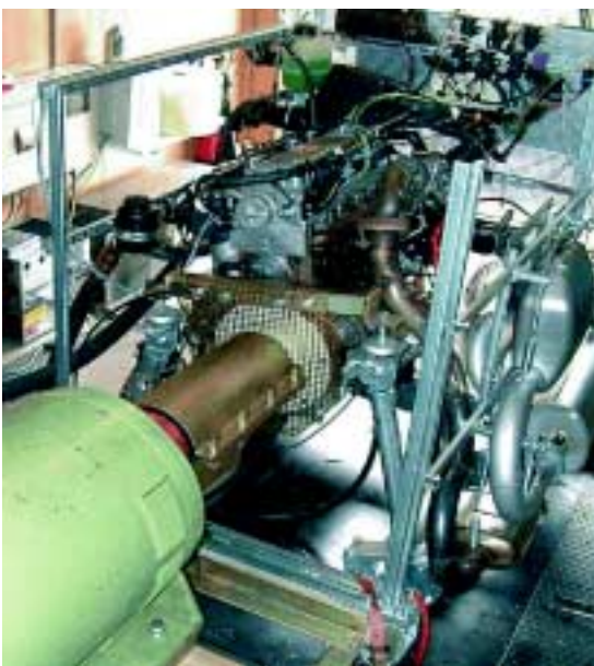
Engine test stand: Opel-DTI diesel engine and asynchronous machine.
