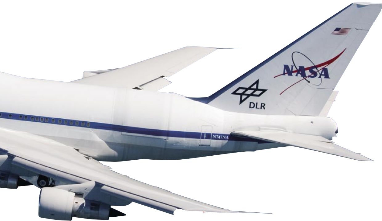
▲ Boeing 747SP during a test flight. The SOFIA infrared telescope is installed in the rear fuselage.
