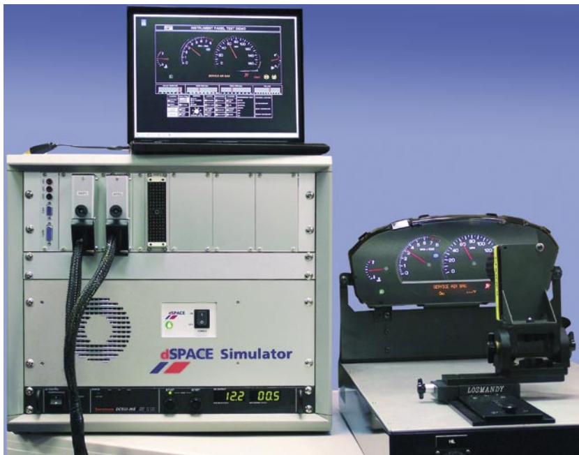
▲ The camera (right) "observes" the instrument cluster and passes the signals on to the HIL simulator.
