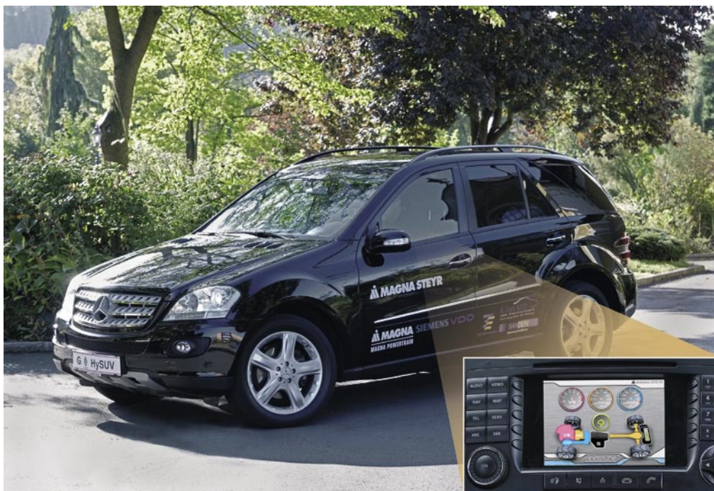
▲ Hybrid driving experience with the demo vehicle HySUV (a modified Mercedes ML350): The display shows the driver and passengers the torque flow of the three propulsion units.
