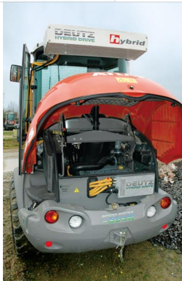
Externally, the only part that differs from the standard wheel loader is the roof-mounted lithium ion battery.
