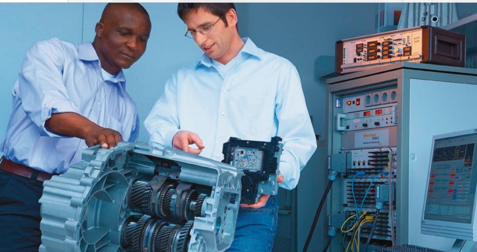
The double-clutch transmission combines the energy efficiency of a manual transmission with the comfort of torque converter transmission.
