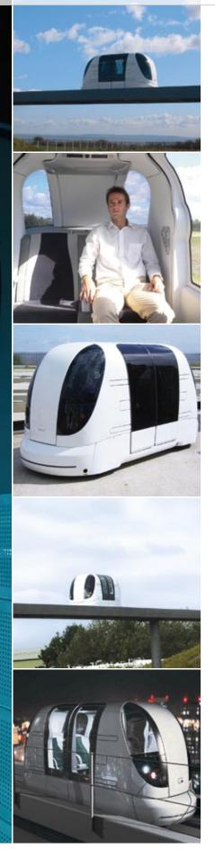
Welcome to the future! From 2009 onward, passengers will be able to travel non-stop across London Heathrow Airport in the ULTra Personal Rapid Transit (PRT) system. This new, environmentally friendly, individual passenger transportation system has been developed by ATS Ltd. The airport operator is using 18 vehicles in the pilot phase – each controlled by its own dSPACE MicroAutoBox as it travels along a 3.8 km guideway network.
