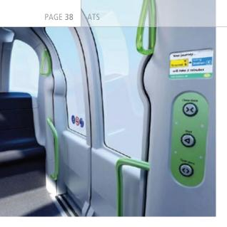
Passengers request their destination at the station and then board their ULTra PRT vehicle. The vehicle travels to the destination non-stop in the slot allocated to it by the synchronous control system.
