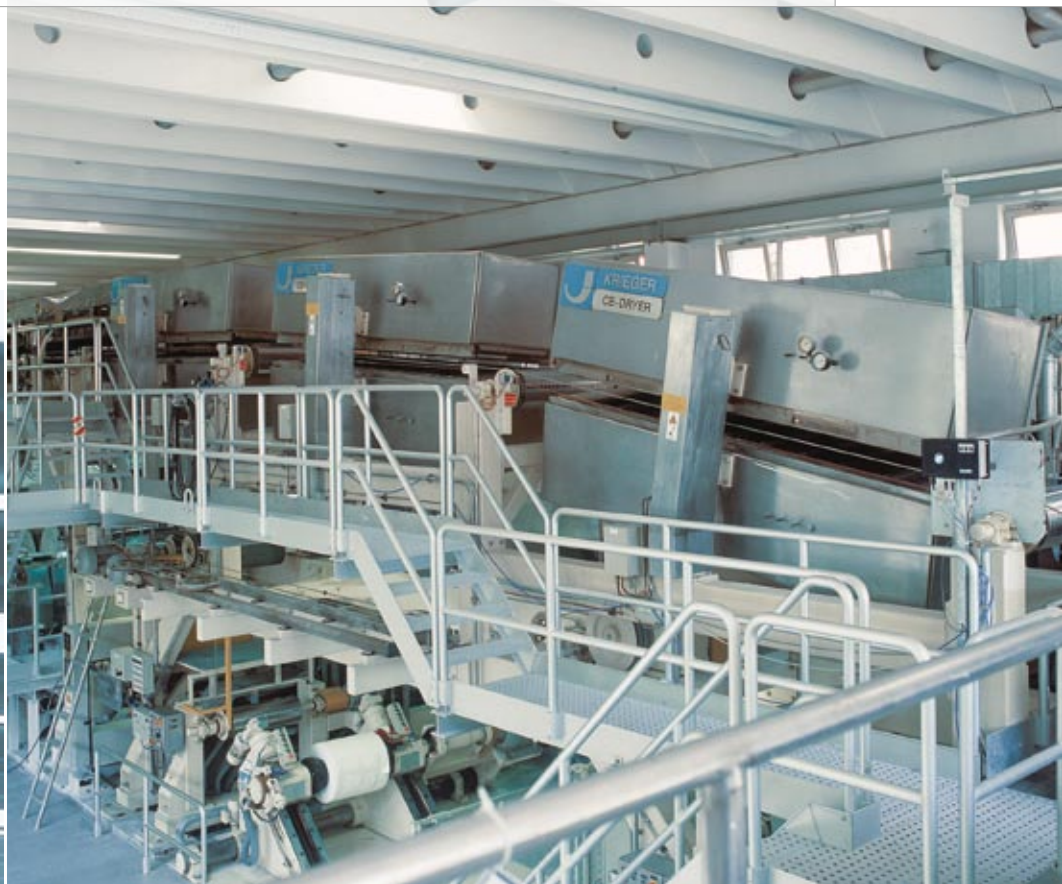
Fig. 1: The VESTRA paper coating system – the pilot coater at PTS, Munich.
