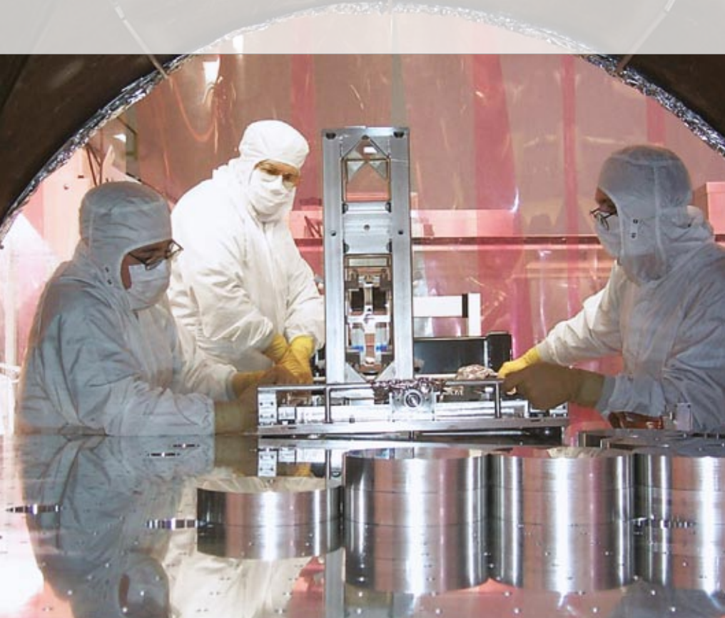
Justage der Spiegel am LIGO. © California Institute of Technology.
