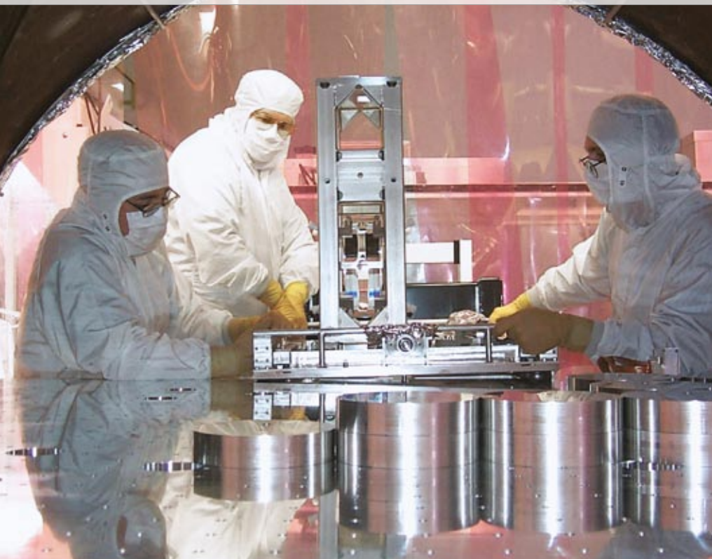
Justage der Spiegel am LIGO. © California Institute of Technology.
