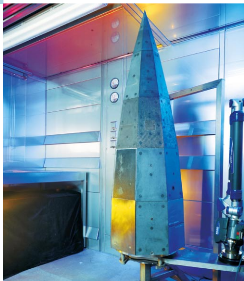
Figure 1: Left: The payload nose cone is just over 2 m long and has flat thermal protection panels.
