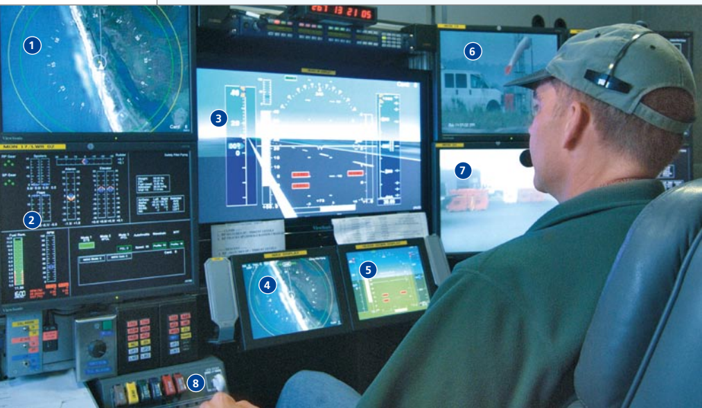
Figure 2: The test pilot's station. Communicating with the UAV by radio, the dSPACE system performs all the ongoing real-time computation tasks so that the test pilot can fly any desired maneuvers realistically from the ground.
