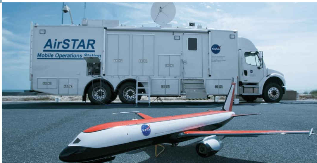
Figure 1: Test flights with the UAV (here in front of the mobile ground station) serve to optimize the functions for flight control computers in passenger planes.
