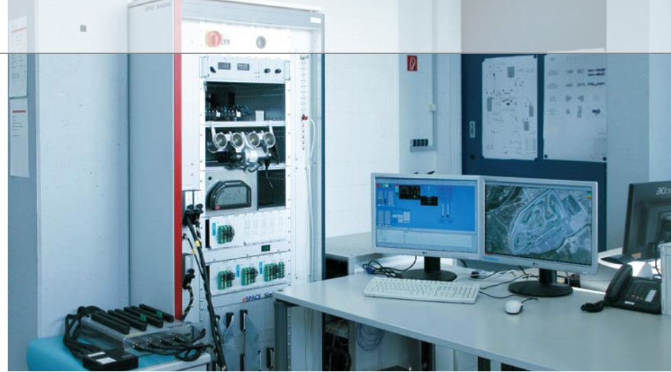
Laboratory test on BMW Motorrad Motorsport's RSM5 engine ECU with the dSPACE HIL test bench.
