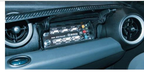
strategies, the hybrid manager is implemented on a modified engine ECU from BOSCH, and the transmission software is implemented on a dSPACE system. Hybridizing the drivetrain necessitates intensive adaptations in the transmission software, such as modifications to the torque interventions and switching sequences.
