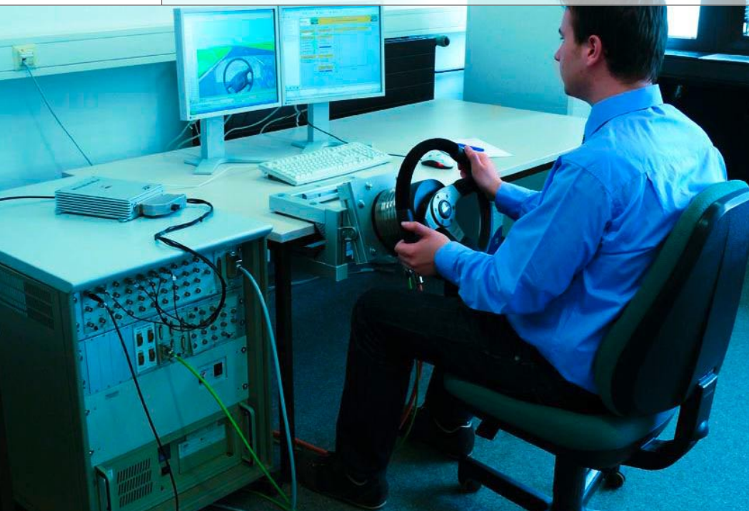
Figure 1: HIL test bench with a feedback steering wheel.
