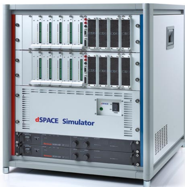
Figure 3: Double dSPACE Simulator Mid-Size.
