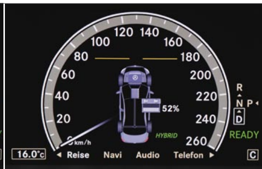
Figure 4c: The vehicle brakes to a standstill (speed 0 km/h; the combustion engine and electric motor are turned off). After this new braking and energy recovery process, the battery's charge has increased to 52 %.
