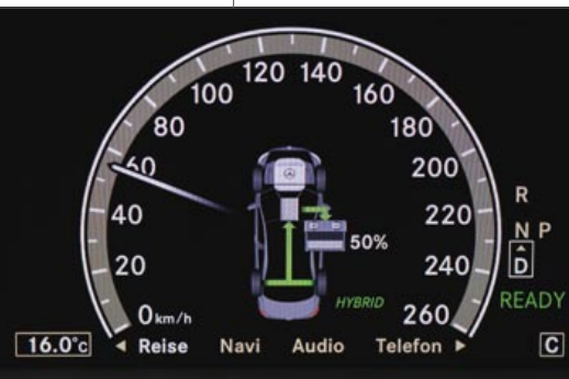
Figure 4a: The vehicle reduces its speed to less than 60 km/h. The electric motor acts as a generator and converts the vehicle's mechanical kinetic energy into electric energy to charge the hybrid battery (energy recovery). The instrument cluster shows this process as a green energy flow towards the battery. The battery is 50 % recharged, and charging continues.
