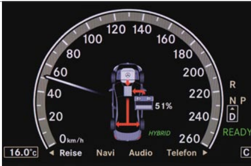
Figure 4b: The vehicle accelerates to over 50 km/h. The electric motor consumes current from the battery and supports propulsion by the combustion engine. The instrument cluster shows the process as a red energy flow towards the wheels. Because of previous energy recovery, the battery charge is now at 51 %.
