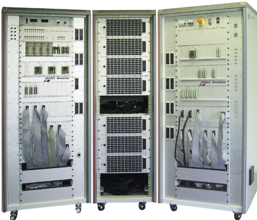
▲ Twin dSPACE Simulators: Renault F1 tests new functions on the new Magneti Marelli Step 11 controller simultaneously in the United Kingdom and France.
