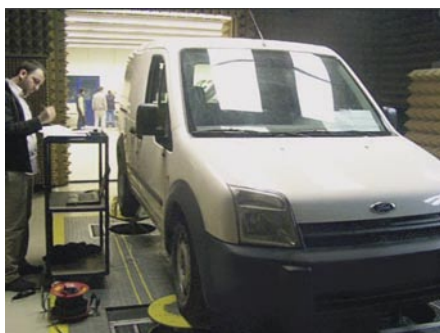
▲ The Ford Transit Connect with semi-active suspension controller is being tested on a four-poster.
