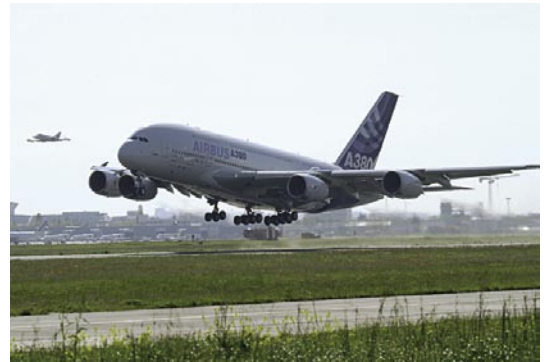
▲ The Airbus A380 during landing: Movable flaps and slats on the wings increase lift and allow the aircraft to fly extremely slowly.
