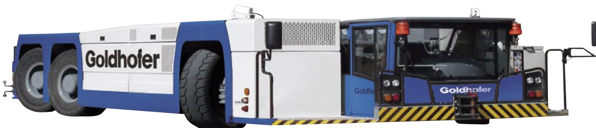
▲ Specially developed for giants like the A380 Airbus, the towbarless AST-1X aircraft tractor from Goldhofer has two Deutz diesel engines.
