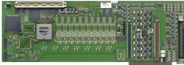
▲ The new DS2202 HIL I/O Board for specific HIL simulations.
