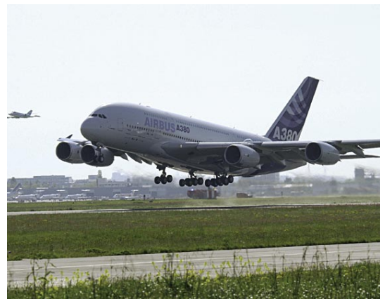
14 The Airbus A380 has a particularly complex system of slats and flaps. Airbus uses a multiprocessor system consisting of modular dSPACE hardware to test them.
