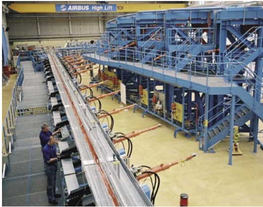
▲ The high-lift test bench for testing the slat and flap system. The airloads of a real aircraft are simulated by hydraulic cylinders.
