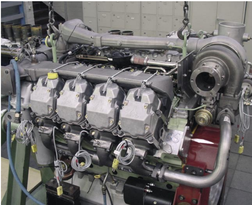
▲ The Deutz TCD2015 V8 4V weighs approx. 1280 kg and has a maximum torque of 3050 Nm.
