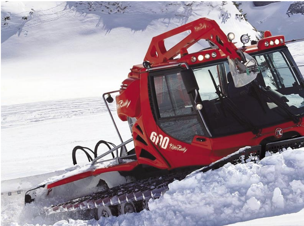
▲ The 11-millimeter-thin steel cable allows work on slopes of 45°.
