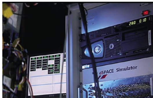
▲ The dSPACE HIL simulator computes the absent truck parts.
