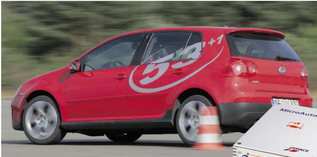
◀ The GTI 53+1 drives round the cones on the test track loop completely autonomously.
