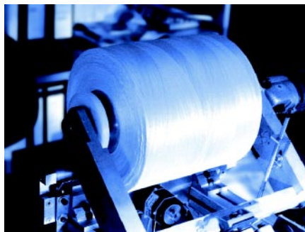
The spool with the thread: length 35 km, diameter 0.6 mm, weight 7 kg, diameter of the spool 250 mm.
