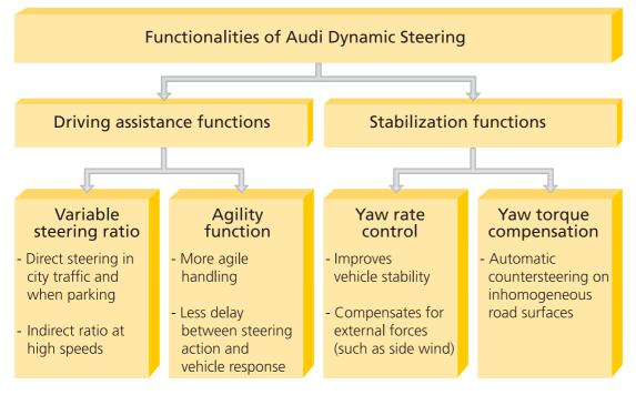
▲ Functional scope of Audi Dynamic Steering. The functions of the steering system allow sporty driving while at the same time providing greater safety in critical situations.
