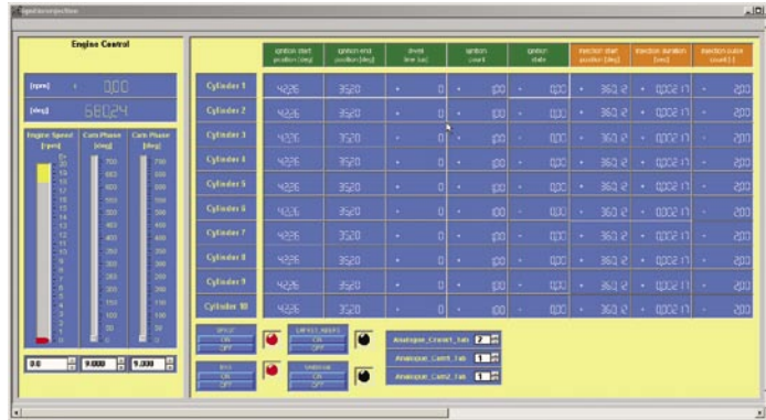
▲ The ControlDesk screen shows the validation of the ignition and injection timing.
