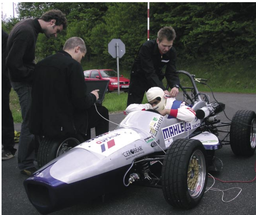
◀ During road tests, data was captured by MicroAutoBox's Flight Recorder, and later evaluated. This allowed errors in the controller model to be found.
