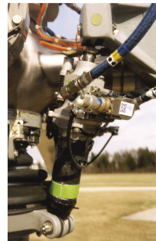
▲ Each of the 4 rotor blades has an actuator for modifying its angle.
