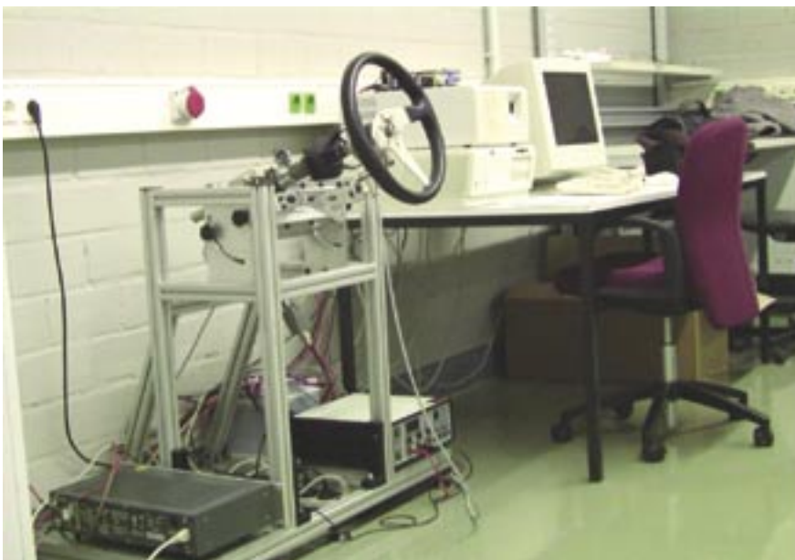
▼ CIL test bench with force feedback actuator.
