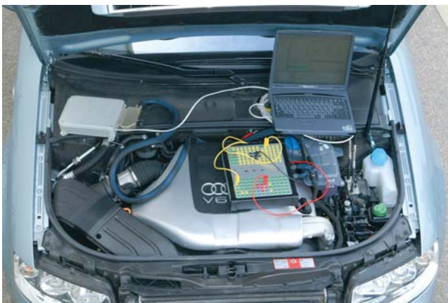
Audi uses dSPACE Prototyper and bypass services for fuel pressure control development.
