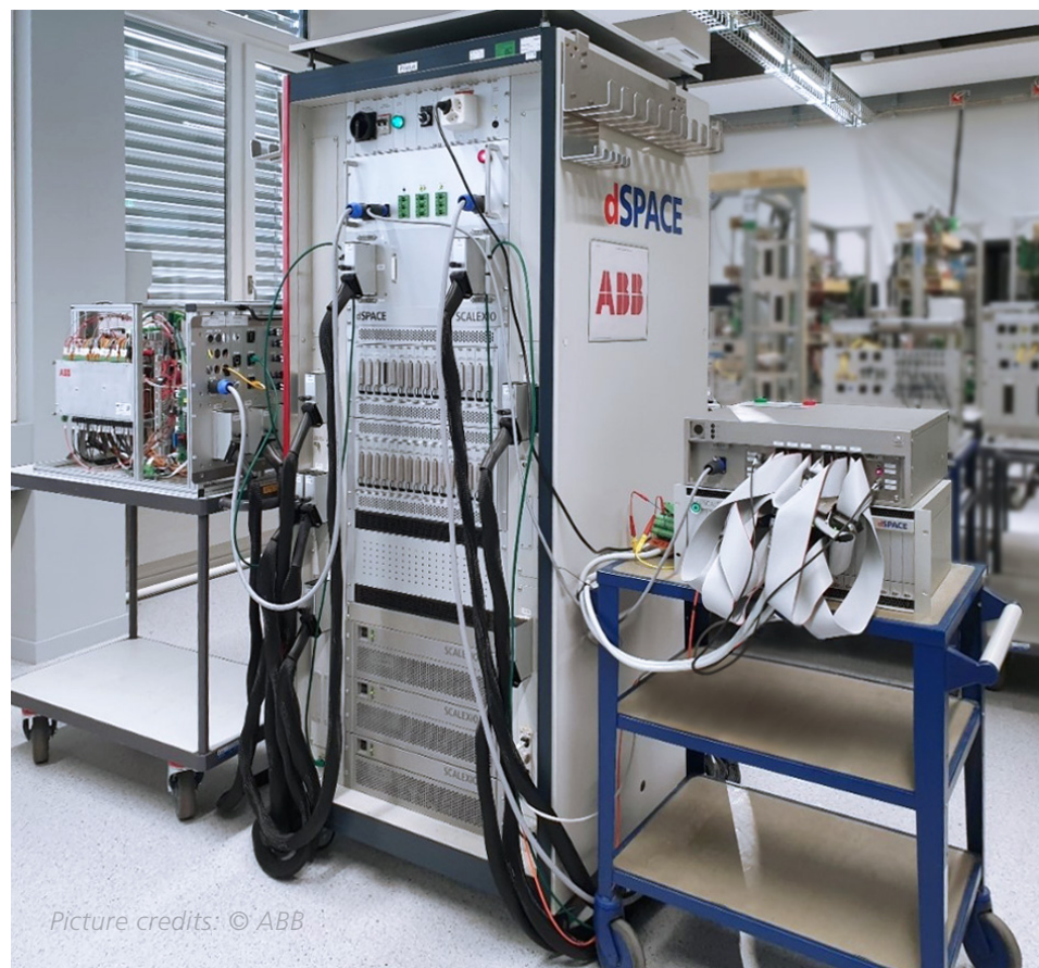
Figure 3: ABB Traction Simulator with dSPACE SCALEXIO systems for combined traction and auxiliary converter simulation.
