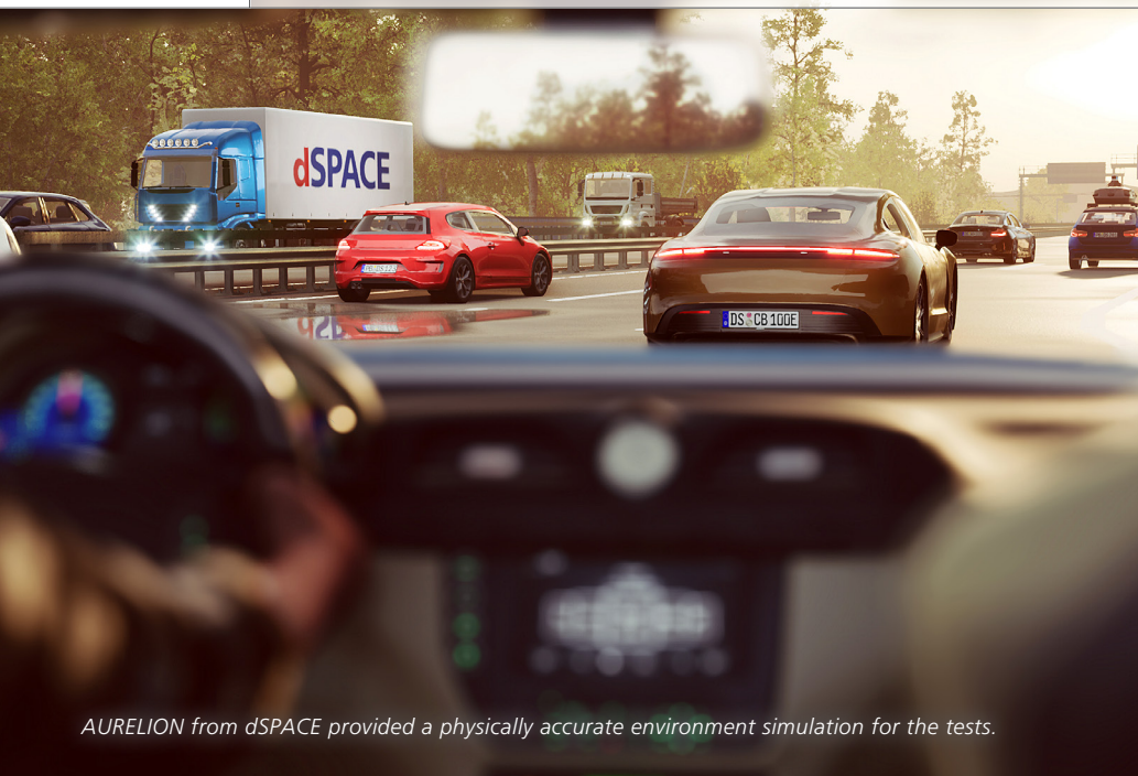
Automotive Simulation Models (ASM) were used to add realistic traffic scenarios and fill the virtual world with vehicles that can be detected by the radar, camera and lidar sensors.
