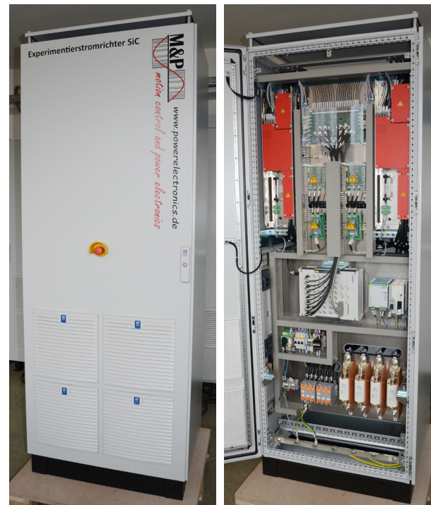
Left: Outer view of the ready-built SiC experiment power converter
