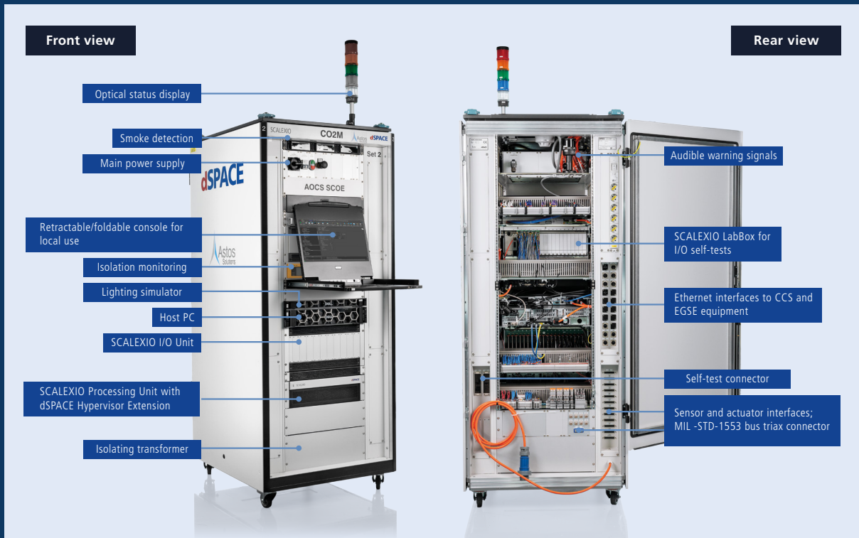
Figure 3: Structure of the dSPACE SCALEXIO system used for the AOCS SCOE. A separate AOCS SCOE will be built for each of the satellites.
