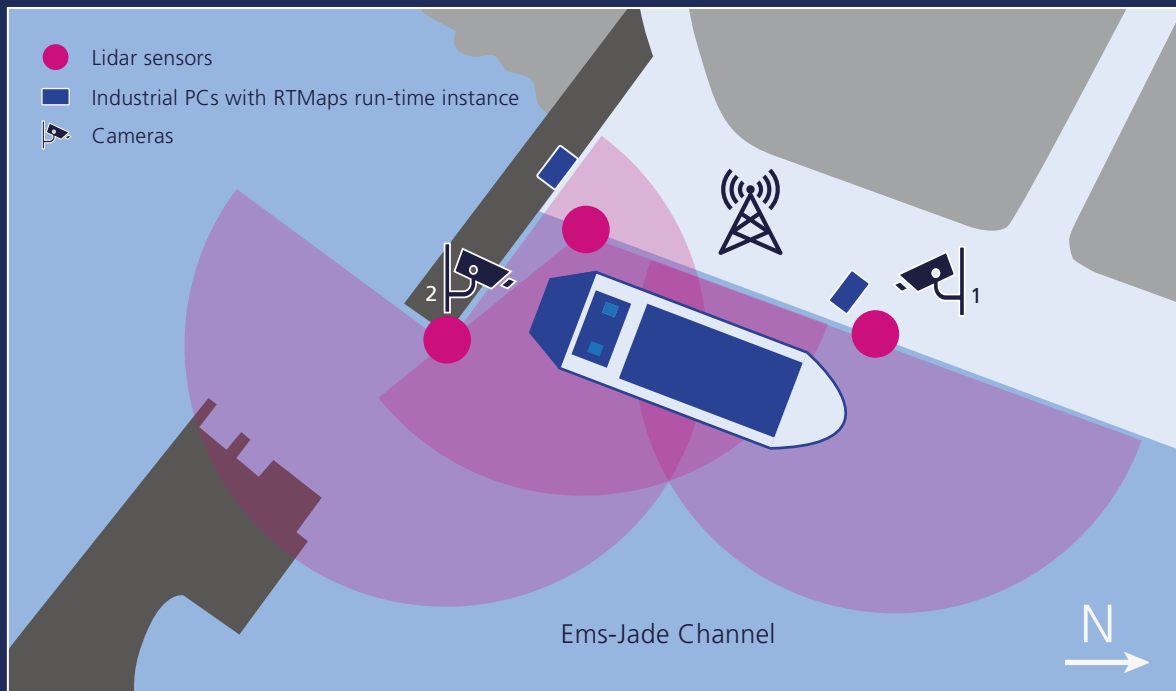
Figure 1: Setup of the SmartKai prototype at Hannover Quay in Wilhelmshaven. The sensors and processors are spatially separate, so synchronization is vital.
