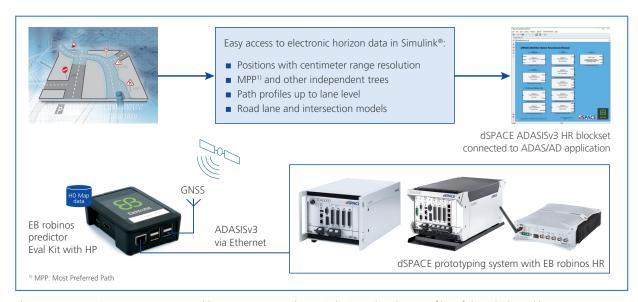
The ADASIS v3 Horizon Reconstructor enables easy access to electronic horizon data (e.g., profiles of the vehicle path) via the standardized ADASISv3 protocol.
