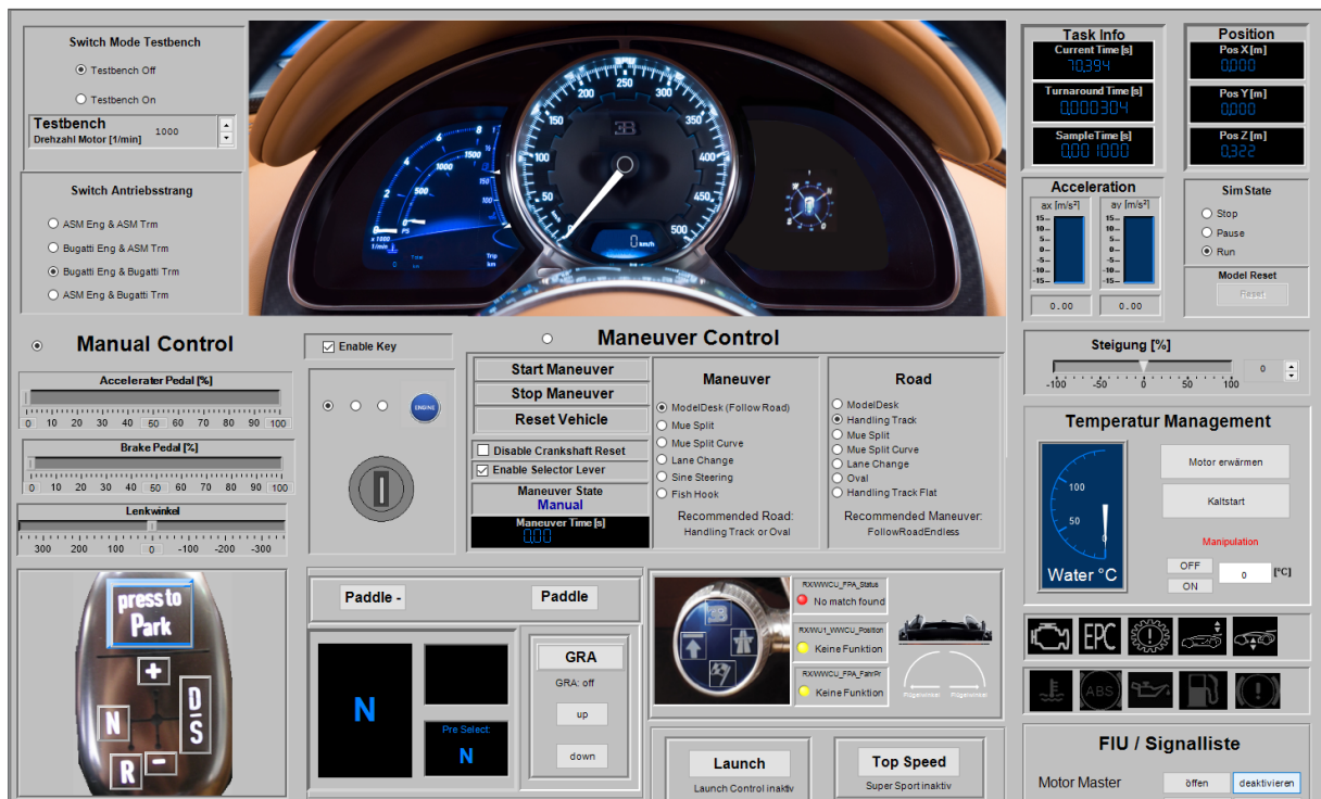
The experiment software ControlDesk sends Bugatti's simulated vehicles on virtual test drives.
