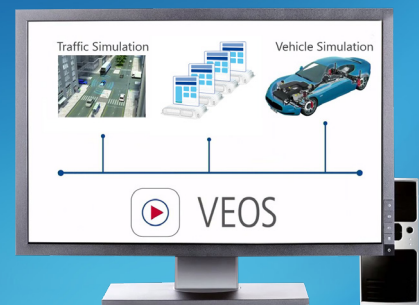
Industry-wide standards are an important prerequisite for virtualizing tests. This involves defining components according to the dSPACE V-ECU approach and integrating them into the VEOS simulation platform together with controlled system models.
