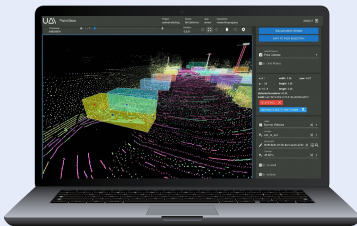
With the web-based UAI tool, an object in a lidar point cloud is accurately marked and then classified.
