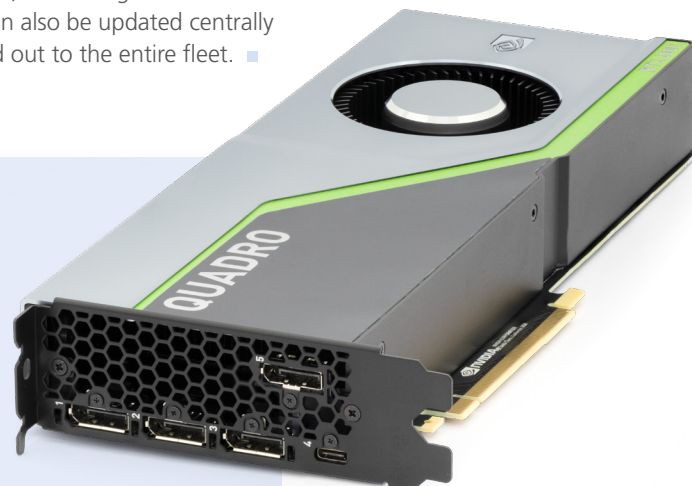
For sensor data preprocessing, AUTERA can be equipped with a powerful graphics card, such as the NVIDIA Quadro RTX 6000.
