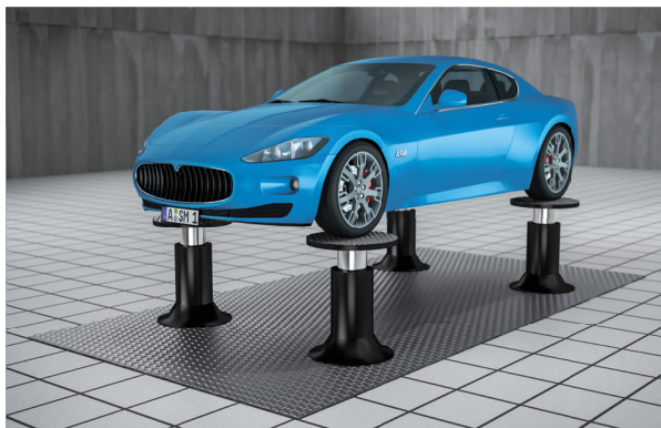
Virtual kinematics and compliance (KnC) test bench.
