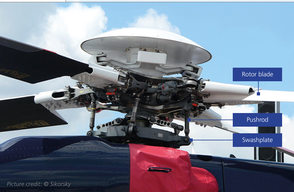
Figure 1: Sikorsky S-92 rotor head with a traditional control system. Hydraulic servos (not visible) are located below the swashplate.
