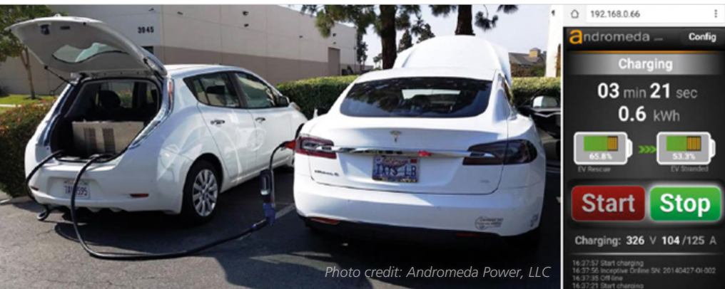
Figure 1: A Nissan Leaf transfers energy to a Tesla Model S through a conductive charging cable. A mobile app communicates with both vehicles and lets the drivers control the charging process.
